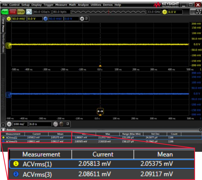
Ultra-low noise at 33-GHz full bandwidth (2.10 mV at 50 mV/div).
