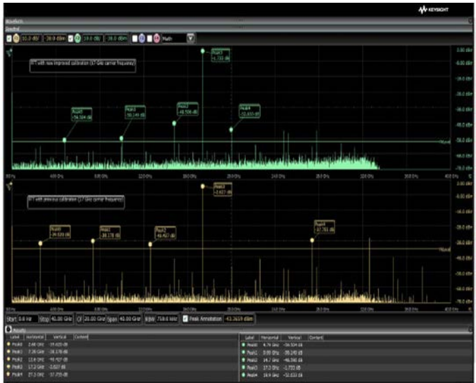
Jitter measurement floor of less than 100 fs (80 fs with 30 GHz input sine wave).
